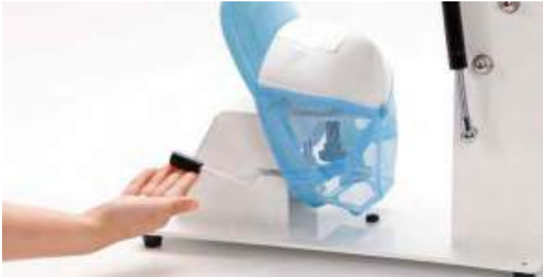
Holding Device It allows the cap to fit the pad for good printing results.
