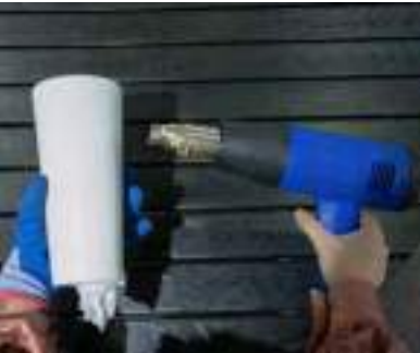
4. Heat the shrink film to make it fit tightly with the substrate;
